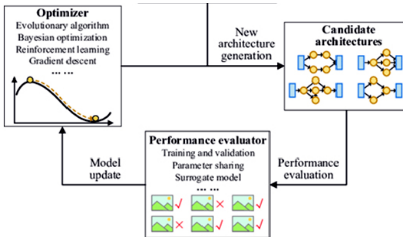
Fig. 14: Architecture selection process (Source: Tian, Y., Peng, S., Yang, S., Zhang, X., Tan, K. C., & Jin, Y. (2021). Action command encoding for surrogate-assisted neural architecture search. IEEE transactions on cognitive and developmental systems , 14(3):1129-1142.)
